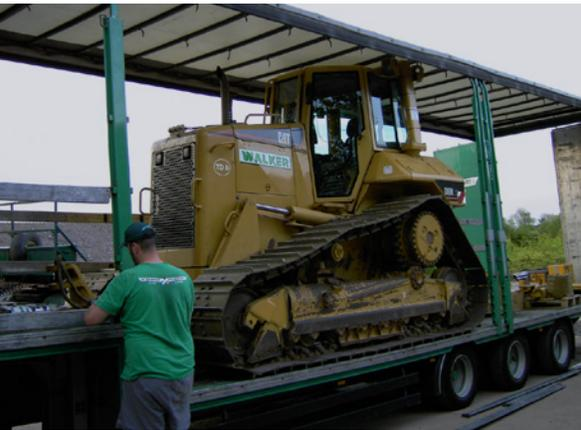
On April 30, 1994, Luis, a new employee aged 25, was helping Jake unload an International Harvester TD9 caterpillar tractor from the flat deck of a truck. As the employee started the tractor and put it in gear, the tractor lurched forward and began to slide sideways off the ramp. The tractor had a ROPS, but he was not wearing a seatbelt. He jumped off to the right, but
